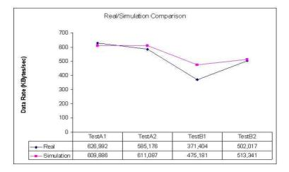
Figure 9: Comparison between real and simulation transmission rates
